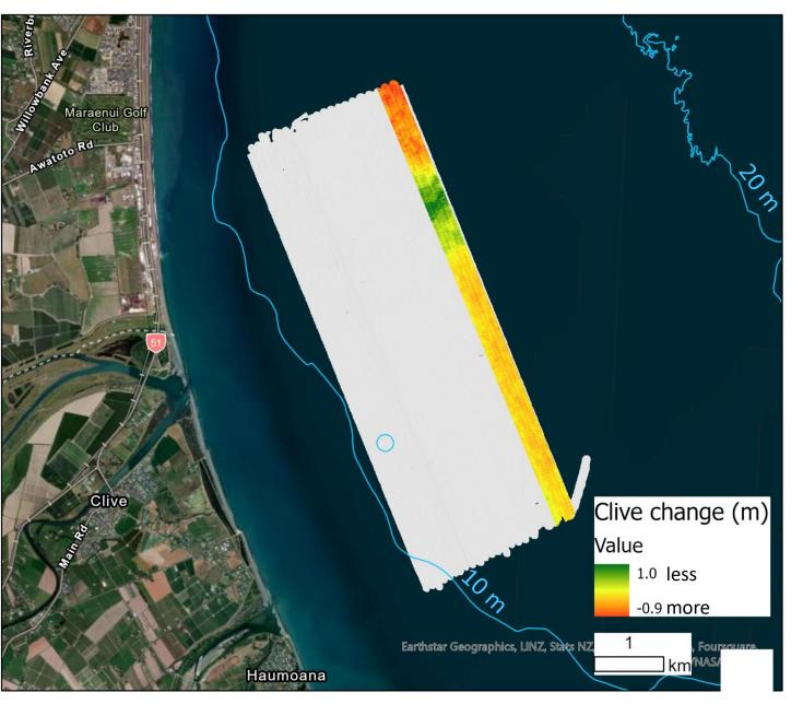
Deposition Erosion of a channel
